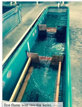
Test flume with two 6in weirs. (NOAA)
