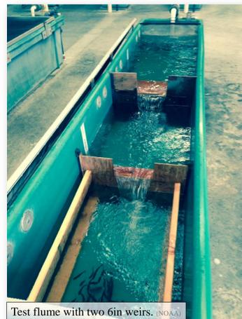
Test flume with two 6in weirs. (NOAA)
