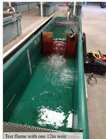
Test flume with one 12in weir. (NOAA)
